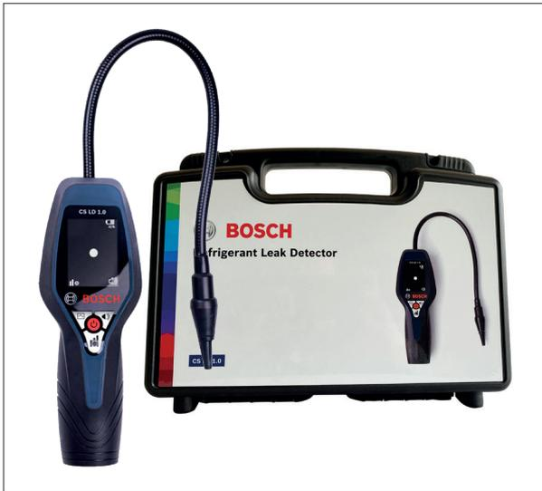
The BOSCH CS LD 1.0 leak detector detects Halogenated CFC, HCFC, HFC, HFO compounds, HC refrigerants such as butane and propane, Tracer Gas (95 %N2/5 %H2 mixture), ammonia.
